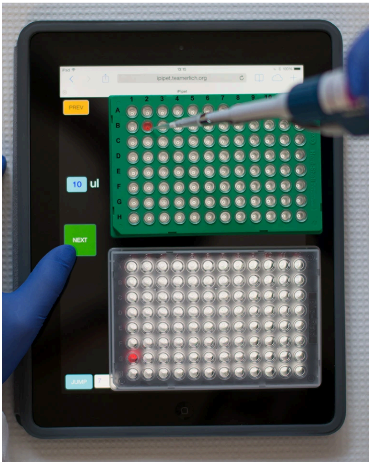
The iPipet app can be used to illuminate sections of a 96-well plate and help researchers to ensure they combine the correct samples. Credit: Dina Zielinski
